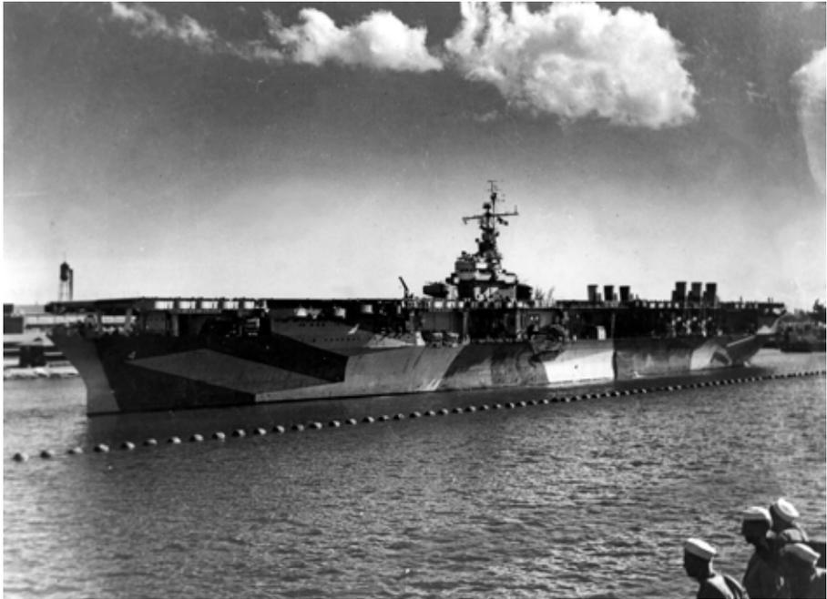
USS *Ranger* after its partial modernization during May to June 1944. Visible is its new radar suite composed of an SM height-finder radar and an SC search radar. The 5"/25 battery was removed as weight compensation for the strengthened flight deck, deck catapult, new radars, and new combat information center (CIC). (NHHHC)
