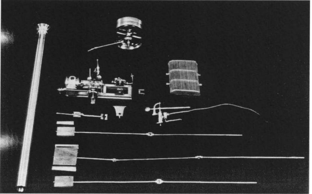
*Figure 9:* Cleaned and newly-fabricated parts. Above are the steam engine and the wheels for the transmission belts that drove the pumps. Below the sluice grating lies the hand pump and at the bottom, three sluices. The funnel to the left is new.
