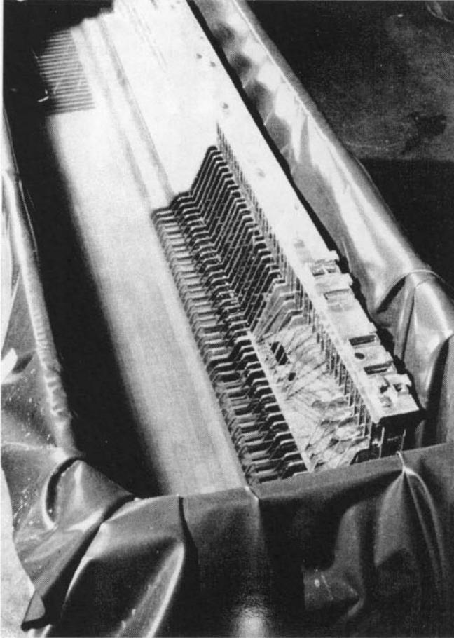
*Figure 12:* The model of the dock sitting in its bath, as yet only half filled.
