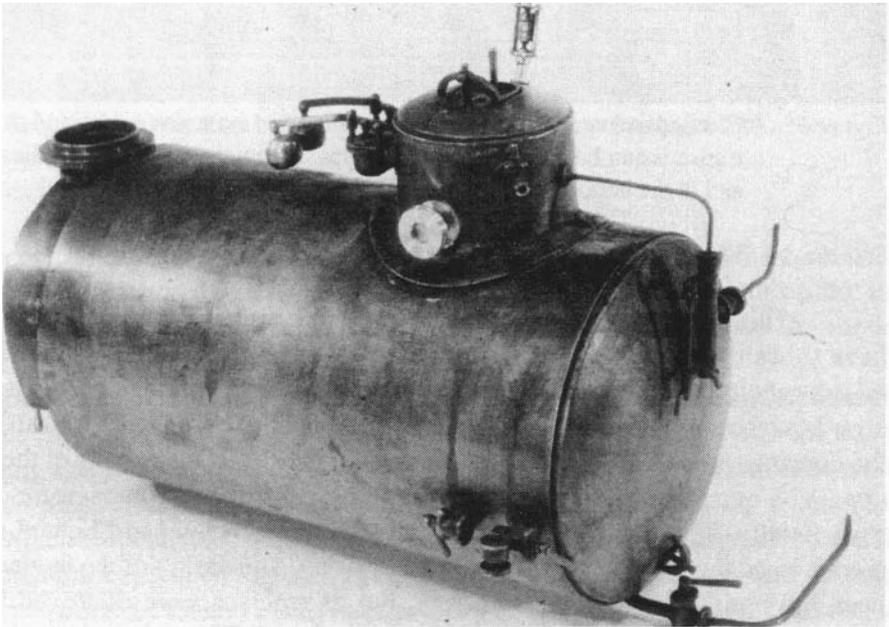
*Figure 8:* The boiler removed from the model before cleaning.
