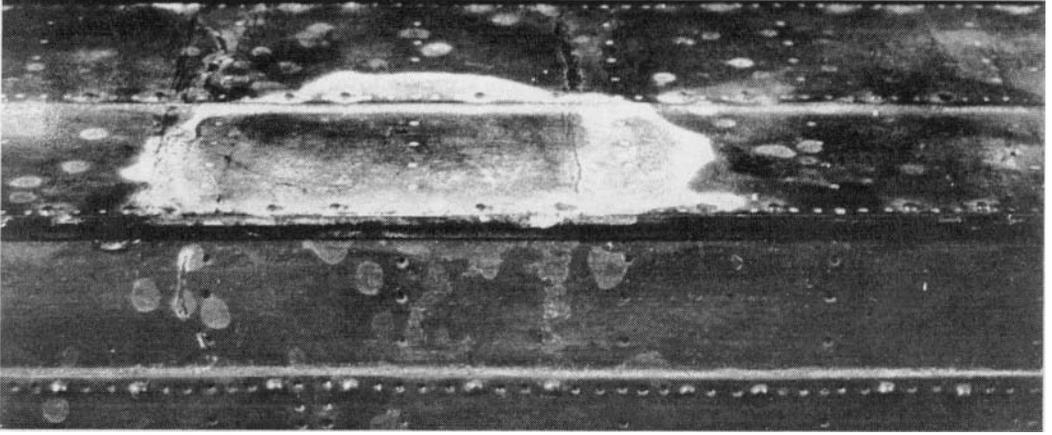
*Figure 11:* Detail of the model of the dock before cleaning, showing the layer of dirt and moisture stains on the upper deck.
